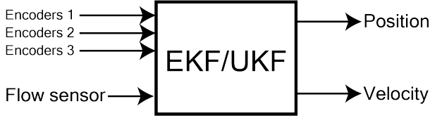
Fig. 2. The Kalman filter framework for state estimation.
