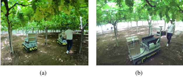
Fig. 5. Human-robot interaction scenarios in the experiment. (a) The human in the shared workspace acts as a dynamic obstacle and activates safety controllers in the robots, forcing them to perform collision avoidance maneuvers and replan. (b) The human collaborates with robot 1 in loading the box, wherein the robot reaches the loading station and awaits human action, following which it continues with rest of its assigned task.
