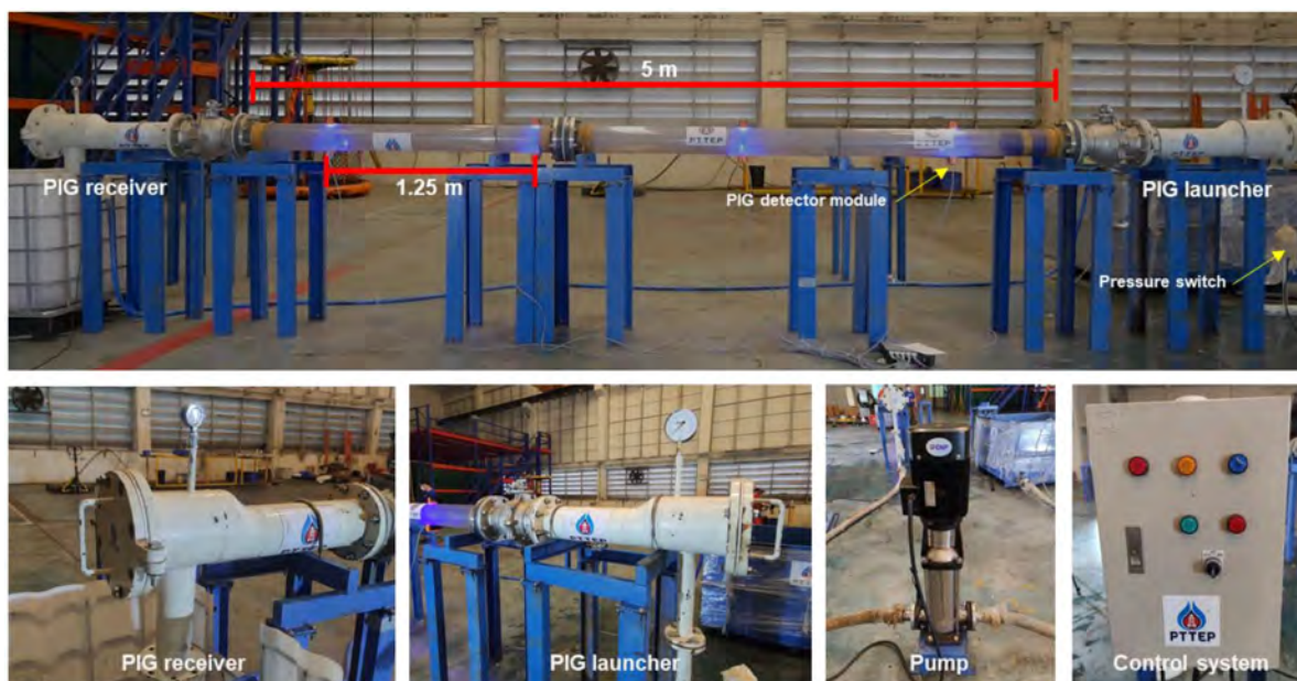
Fig. 13—The experimental setup and testing system of the 3D-printed MC-PIG prototype.
